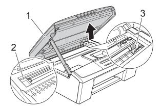
Move the print head (if necessary) to take out any paper remaining in this area. Make sure that jammed paper is not left in the corners of the machine (2) and (3).
